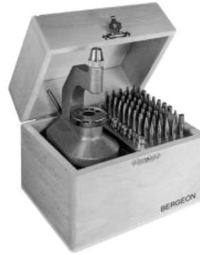
No. 5285-B Ditto. Containing: 50 punches. Dia. 4.7 mm. 10 stakes.
