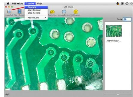
**Delete a Captured image:** Select the captured image in the image scroll list -> press “Del” Key of keyboard to delete it.
