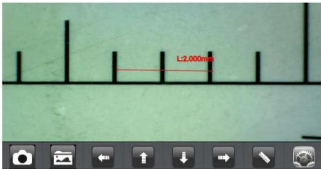
Now the calibration is completed. Click on screen again, you can make measurement features accurately on the live video at this same focus. (Please, don't adjust again the “Focus & Magnification wheel”). If the new photo object is not in focus, please only adjust the distance between the microscope and the object until the photo is clear. The measurement data can be saved inside the taken photo.
