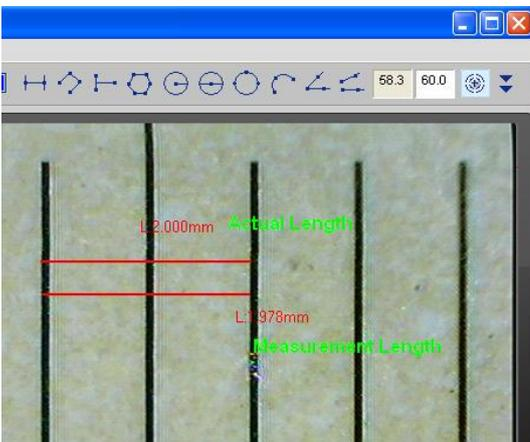
The software will automatically calibrate the scale of magnification and will show the calibrated scale of magnification at the right-hand box of calibration button
