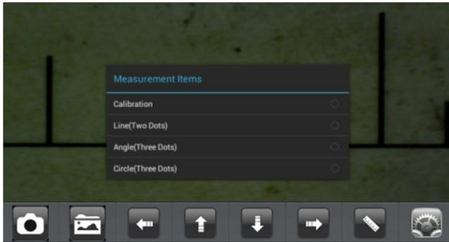
Use the enclosed calibration ruler as to-be-observed object. Bring photo into focus by turning the “Focus & Magnification wheel”; Click on
