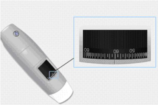
1. To calibrate, select a known measurement standard, such as a ruler, as to-be-observed object.
