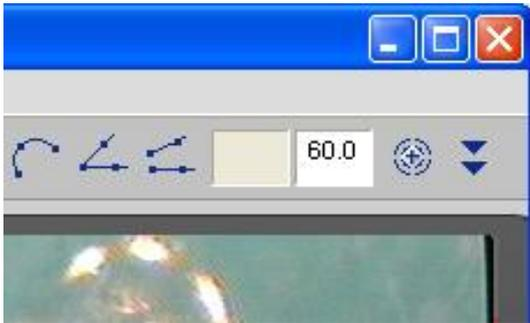
4. Enter the scale value in the "Scale" box in the right-hand scale box of the screen
