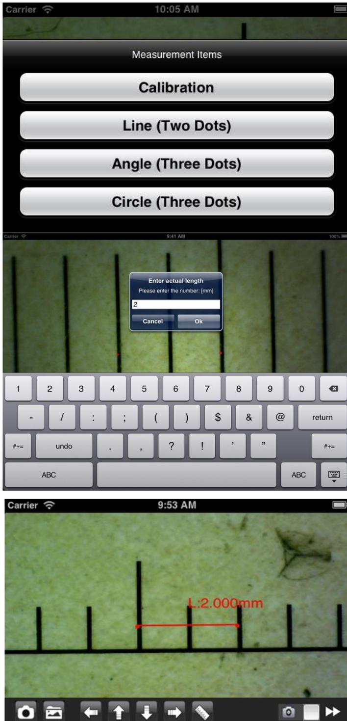
Use the enclosed calibration ruler as to-be-observed object. Bring the image into focus by turning the "Focus & Magnification adjustment wheel";
