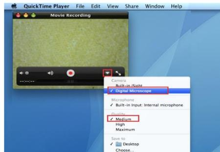
Click on the dropdown arrow at the bottom right of the “New Movie Recording” window. Make sure the USB Digital Microscope is the selected Camera and that Quality value is set to Medium, as shown on the left.
